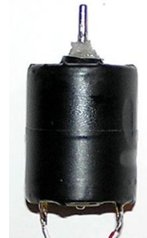
Figure 2.6-4: Petroleum Jelly Placed at the Base of a Motor's Shaft
