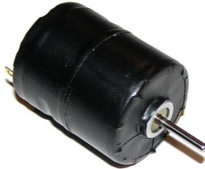
Figure 2.3-1: A Motor Sealed with Electrical Tape
