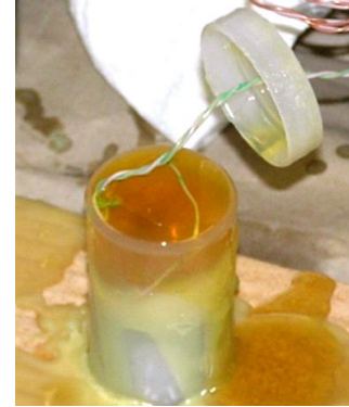
Figure 2.6-10: Filled Housing Ready to Cap
