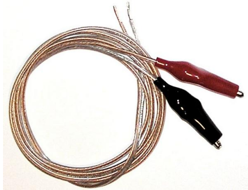
Figure 3.3-1: Completed Power Cord
