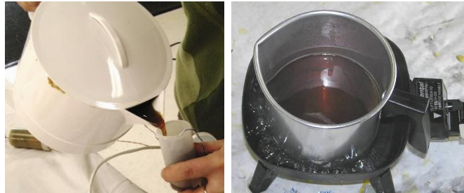
Figure 2.6-3: Wax Melted in an Electric Heating Pot or in a Metal Cup Placed in an Electric Skillet (with Water to Help Regulate the Temperature)
