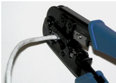
Figure 3.2-8: RJ45 Connector Plug in the Crimping Tool Cavity
