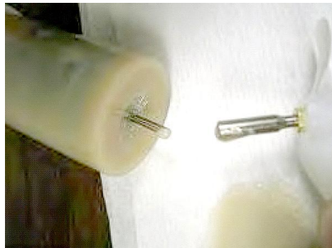
Figure 2.7-8: Epoxy Placed on Motor Shaft Tip and Hollow End of the Shaft Coupler
