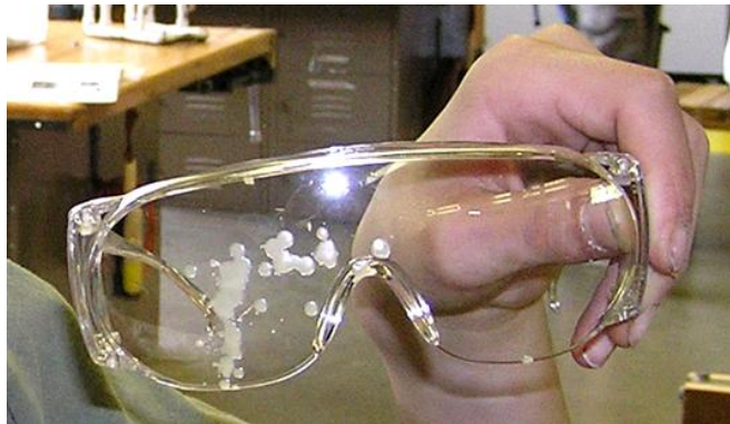
Figure S-1. Wax Squirted onto a Student's Safety Glasses
