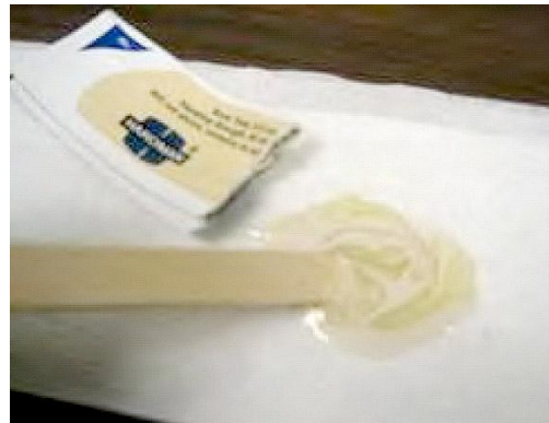
Figure 2.7-4: Stirring the Epoxy Until Its Color is Uniform
