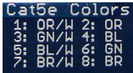
Figure 3.2-4: Connector Wire-Color Sequence Printed on the PCB
