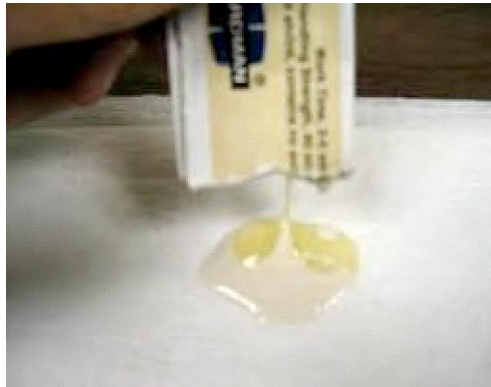
Figure 2.7-3: Two-Part Epoxy Squeezed Out onto a Piece of Paper
